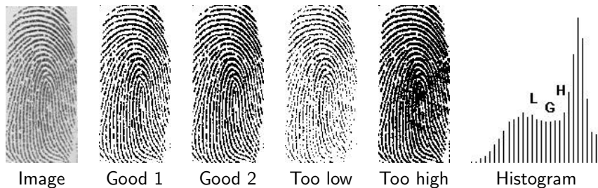
Thresholding a fingerprint image. In the histogram, positions of good (G), too low (L) and too high (H) thresholds are shown.
