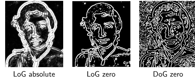
Examples of edge detection by 15 \times 15 LoG and DoG operators. 'LoG absolute' is absolute value of filter output: dark lines are contours. 'LoG zero' was obtained with removal of weak edges, 'DoG zero' without removal.
