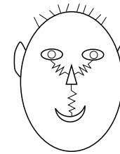
Representing a face template as a set of flexibly connected subtemplates.
